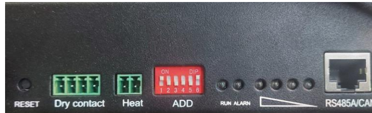
Figure 2: Image of BMS orientation (master BMS DIP setting).
